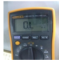
Figure 5-4.7: Measuring resistances between compressor terminals and ground
