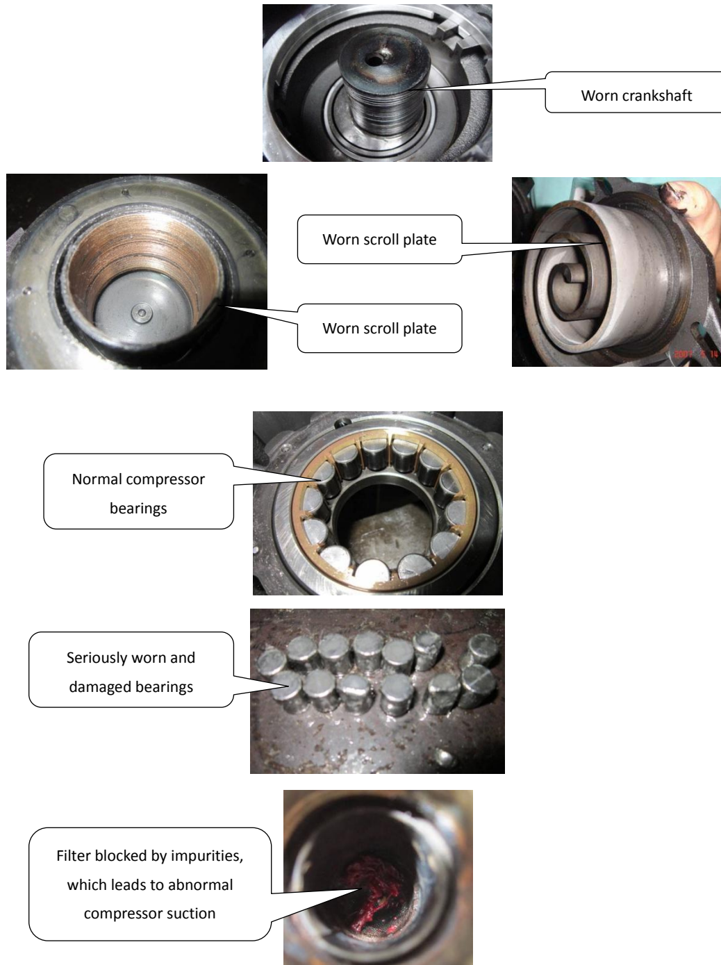
Figure 5-4.17: Effects of spoiled compressor oil
