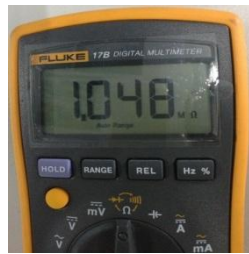
Figure 5-4.6: Measuring resistances among compressor terminals
