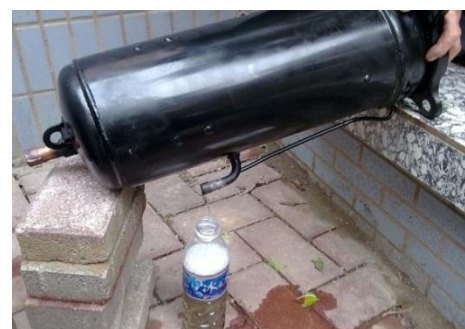
Figure 5-4.14: Draining oil from a compressor
