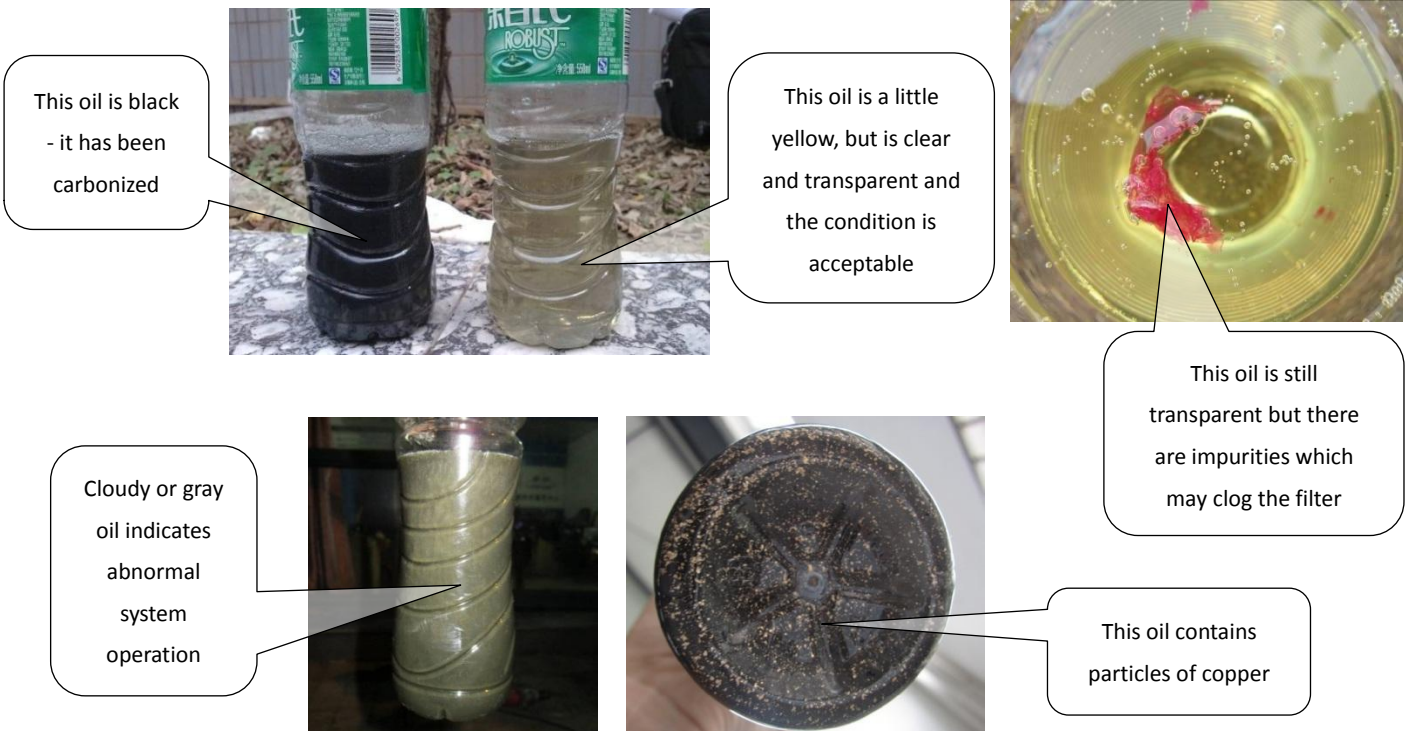
Figure 5-4.16: Inspecting compressor oil
