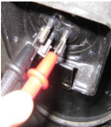
Figure 5-4.6: Measuring resistances among compressor terminals
