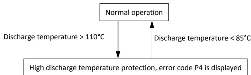
When the discharge temperature rises above 110°C the system displays P4 protection and the unit stops running. When the discharge temperature drops below 85°C, the compressor enters re-start control.
