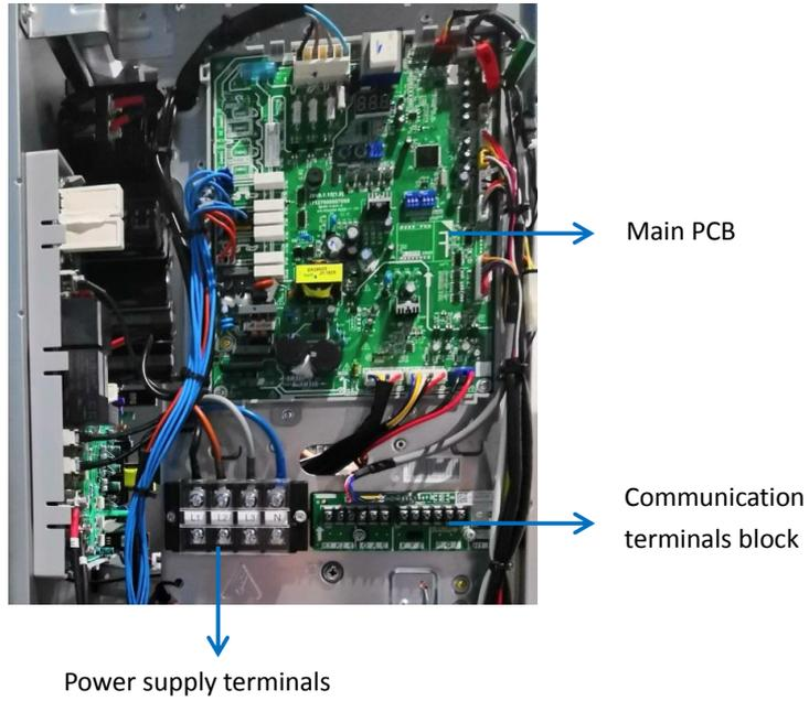
Figure 5-1.2: Rear view of electric control box
