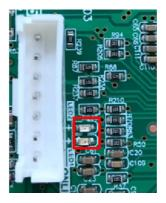
$3. \quad \text{Check the power supply for the compressor drive module, the normal voltage L2 and N (CN4/CN6) 198v-242V.}\\$
