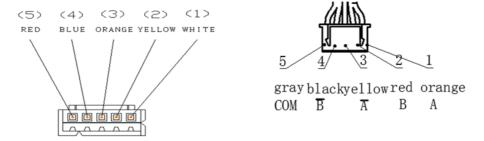
Figure 6-2.3(b): EEVC coil wiring terminals
