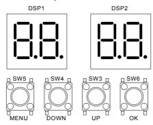
Close liquid stop valve and high pressure gas stop valve of all outdoor units, Meanwhile, the digital display will display "r001";
