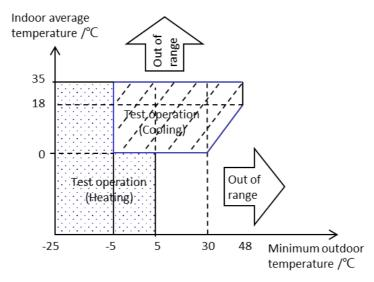
If it is out range of test operation, the outdoor unit displays the fault code "U21 or U22 or U23".
