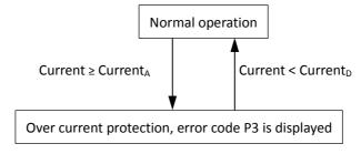
Table 3-6.1: Current limitation for compressor inverter modules
