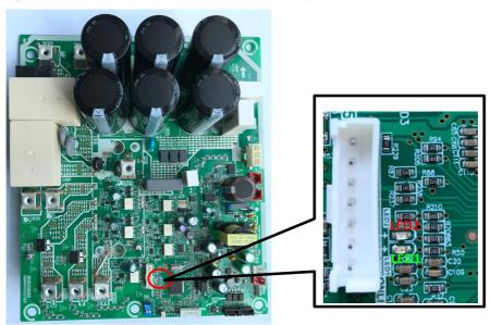
Figure 6-2.5: 14-18HP LED indicators LED1 and LED2 on compressor drive module
